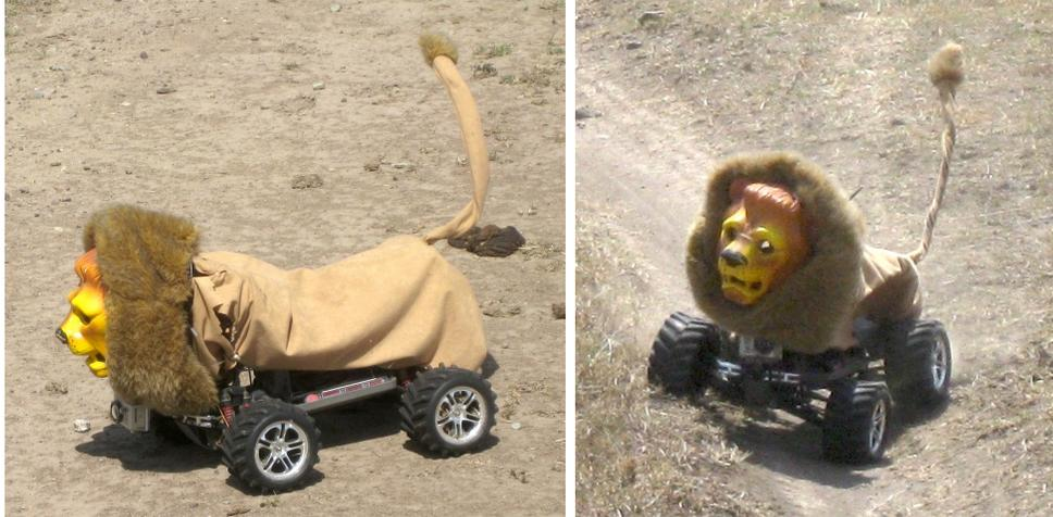
Figure 5.1: The “robo-lion” remote-controlled artificial predator device, measuring approximately 40 cm wide and 60 cm long. Left: side view. Right: front view.
