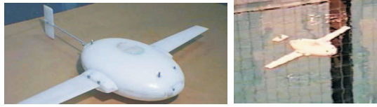
Figure 2.1: Experimental, laboratory-scale underwater glider ROGUE.
