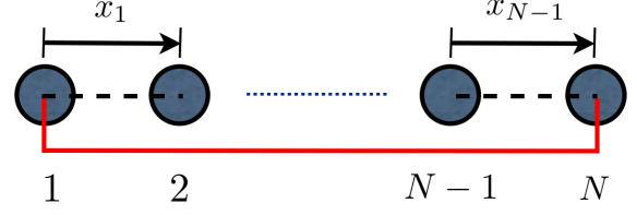
Fig. 2. Shape coordinates along the line. The dashed lines represent cable interconnections and the solid line represents a strut.
