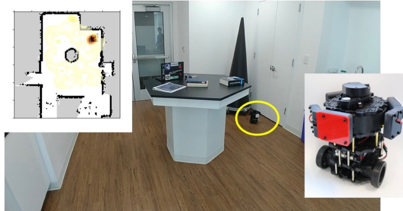
FIG. 1. Image of gamma inspector bot searching room for gamma sources located under a mock warhead. Insets show (left) the occupancy map created using SLAM overlaid with the measured activity (red indicating higher activity) using estimated measurements given by Gaussian Process (GP) Regression (see Section 4) and (right) a larger view of the gamma inspector bot.
